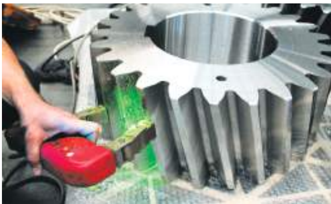
Magnetische Partikuletests / Magnetic Particle Inspection
